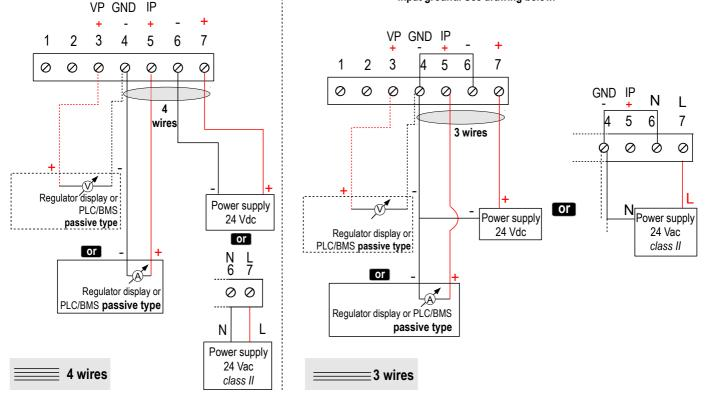
For CP114/115 - PO models and CP114/115 - PN models with 4-20 mA output - passive :
